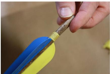
Step 5 – Repeat the whipping on the other end of the vanes. After you have trimmed the ends from the whipping, you can apply a drop of glue to prevent the whipping from loosening.
